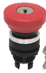
Push Key Mushroom. Manual push "In". Automatic latches "In". Turn key clockwise to release. Spring return. Key withdrawable "Out" position only. Red only.
